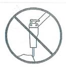
**Blank Firing.** Special care has to be taken not to carry out blank firing. A blank firing may cause Tie Rods' breaking. These are parts which keep together the various components of the breaker. Furthermore it may cause Retaining Pins' and Tools' breaking. Thus you have to disconnect the power supply to hammer at the exact moment of rock breaking.
